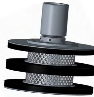
Figure 8: Acoustic Nozzle Exterior View
