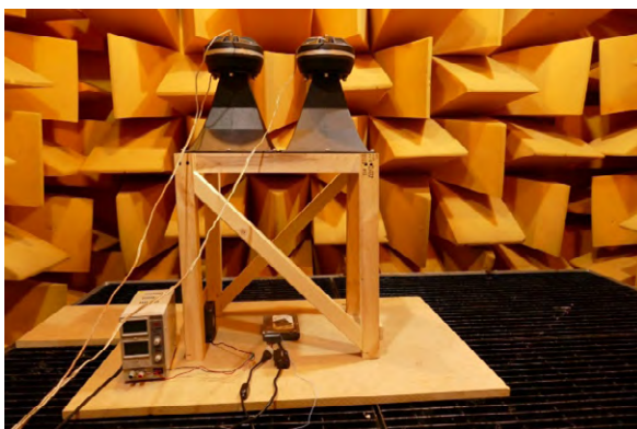
Figure 2: Photograph of the test set-up showing the HDD on an MDF board in the anechoic chamber at Michigan Technological University with the speakers placed 0.5 m above the HDD (left). The surface mount microphone, a fan used for cooling the HDD and the USB 3.0 cables used for performance test (right).
